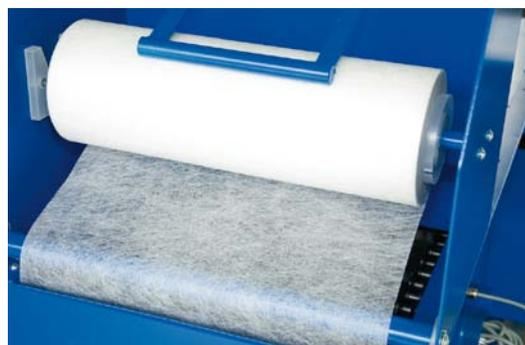
Filter fabric in gravity band filters
