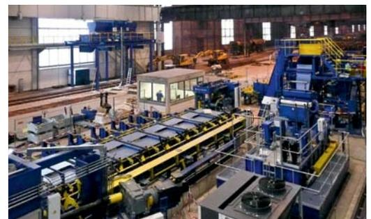
Central chip system for steel bar peeler with vacuum sluice and silo storage for the filling of railway freight cars
